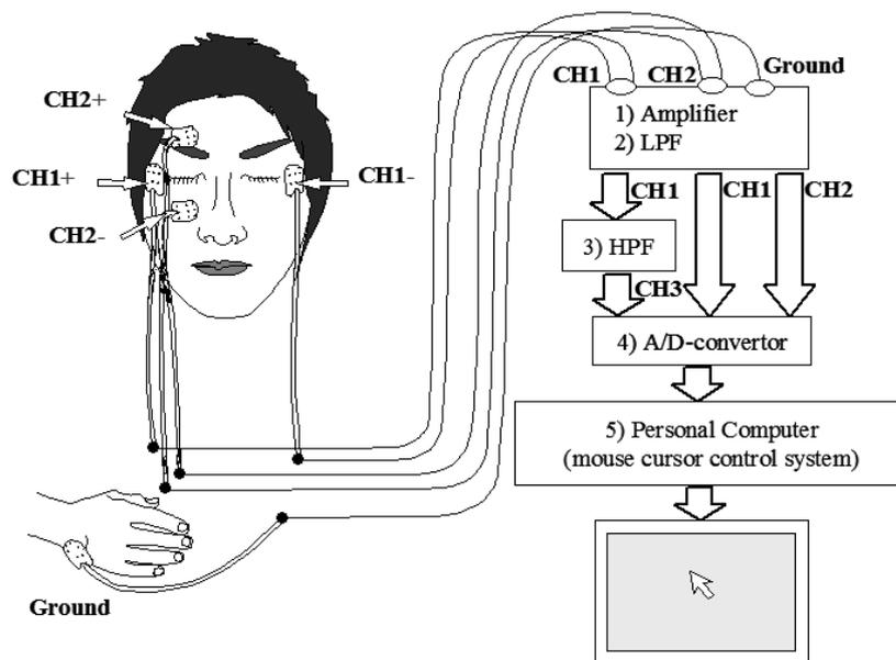
Fig 1: The Mouse Cursor Control System using EOG
