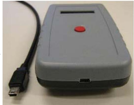
The command summary for this reader is identical. Especially large amounts of data can be transferred more rapid, and due to the higher clock speed of the processor, searching data is done quicker. The battery voltage is realtime measured and shown on the LCD.
